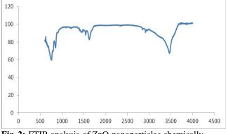
Fig. 2: FTIR analysis of ZnO nanoparticles chemically.
