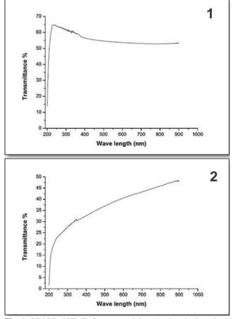
Fig. 1: UV-Vis-NIR ZnO nanoparticles (1) chemical method, (2) aqueous hydrolysis.
