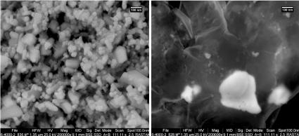
**Fig. 6:** SEM image of ZnO NPs (A) aqueous hydrolysis (B) chemical.
