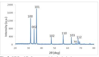
Fig. 5: XRD of ZnO nanoparticles hydrolysis.
